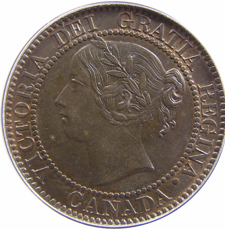
Figure 3 The DP#1 Obverse. Note the die cracks at 2:30, 6:00, 9:00, and 11:00.
